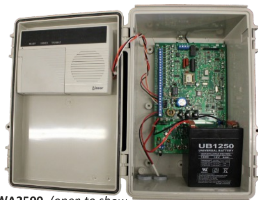
WA2500, (open to show keypad and control panel.)
